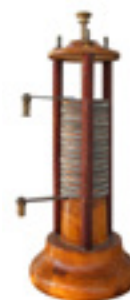
Volta's battery is the first, rudimentary generator of direct current
